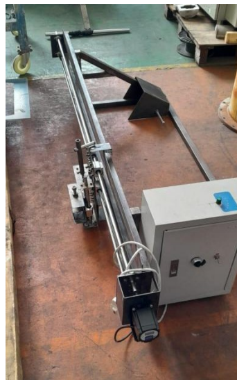
Gambar 5. Realisasi alat bantu gerak plasma cutting
