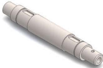
**Gambar 7.** Model poros Conveyor Unit
